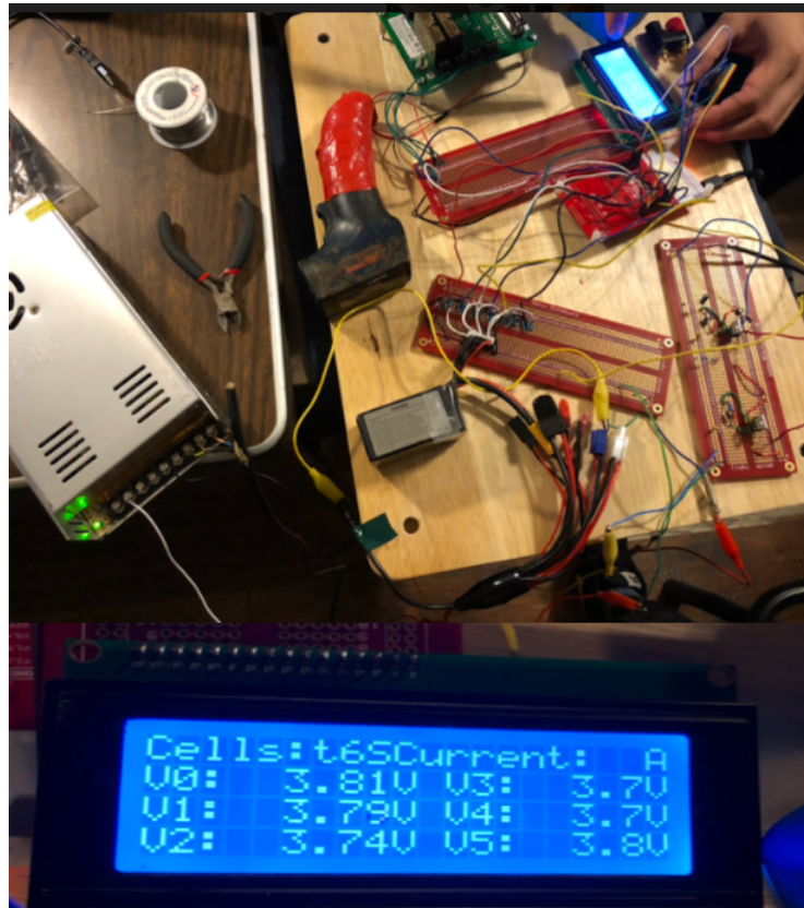
Figure 8. Hardware setup for fault detection test
